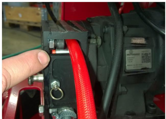
**IMPORTANT:** The pump will automatically stop if door is left open. Keep door closed during operation.
